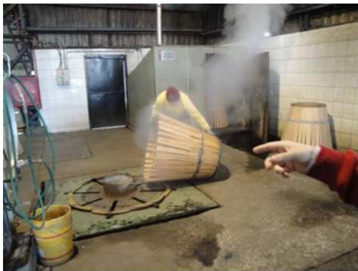
Figure 1. Wine barrel being assembled at a cooperage in Chile
